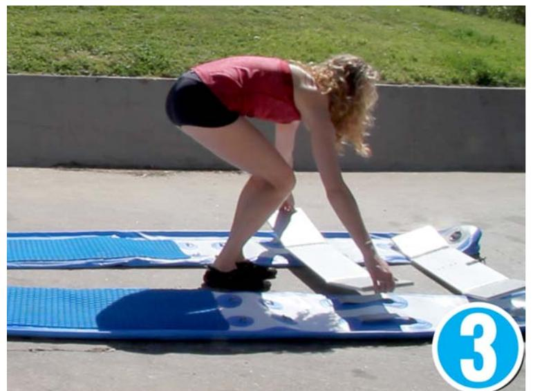
Slide each cross bar into the deflated hulls' straps. On the front and rear cross bars, screw the retainer bars into threads ends of the cross bars, clamping onto the straps.
