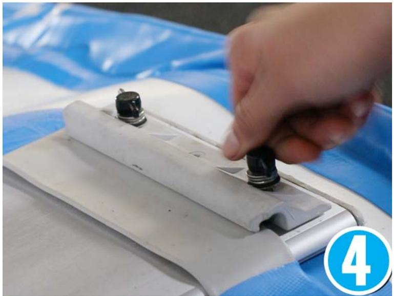
Remove the covers from the air valves and turn the air valve stems until they pop up in the "no-air flow" position.
