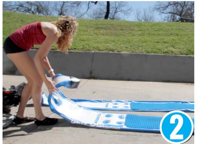
Place the cross bars in the correct order from front to back on the hulls and space the hulls apart to fit.
