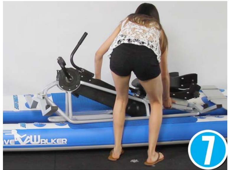
Align the frame assembly support bars between the mounting rings on the hulls and attach the frame assembly to the hulls with the cinch straps, making sure they are snug. Wrap the strap ends under, so they don't come loose during use.
