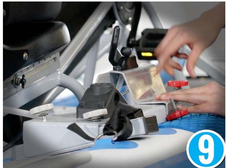
Attach the rudder assembly to the rear cross bar using the two attached screws. Remove the rudder pin from the rudder bracket by rotating the circular cotter pin.
